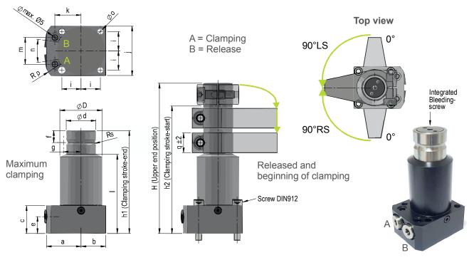
For size 1 - "n" is the angle. For size 2-3 it is the gap between both ports.
